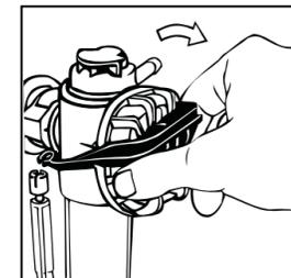
**LOW PRESSURE APPLICATION:** If it takes longer than 4 minutes to refill your cistern, you can increase the flow of water by removing the flow restrictor. **IMPORTANT:** Always clear any debris from water line before installation.
